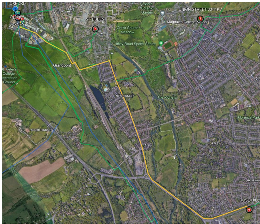
Figure 6: Load Shift Rose Hill to Osney BSP, new cable route
