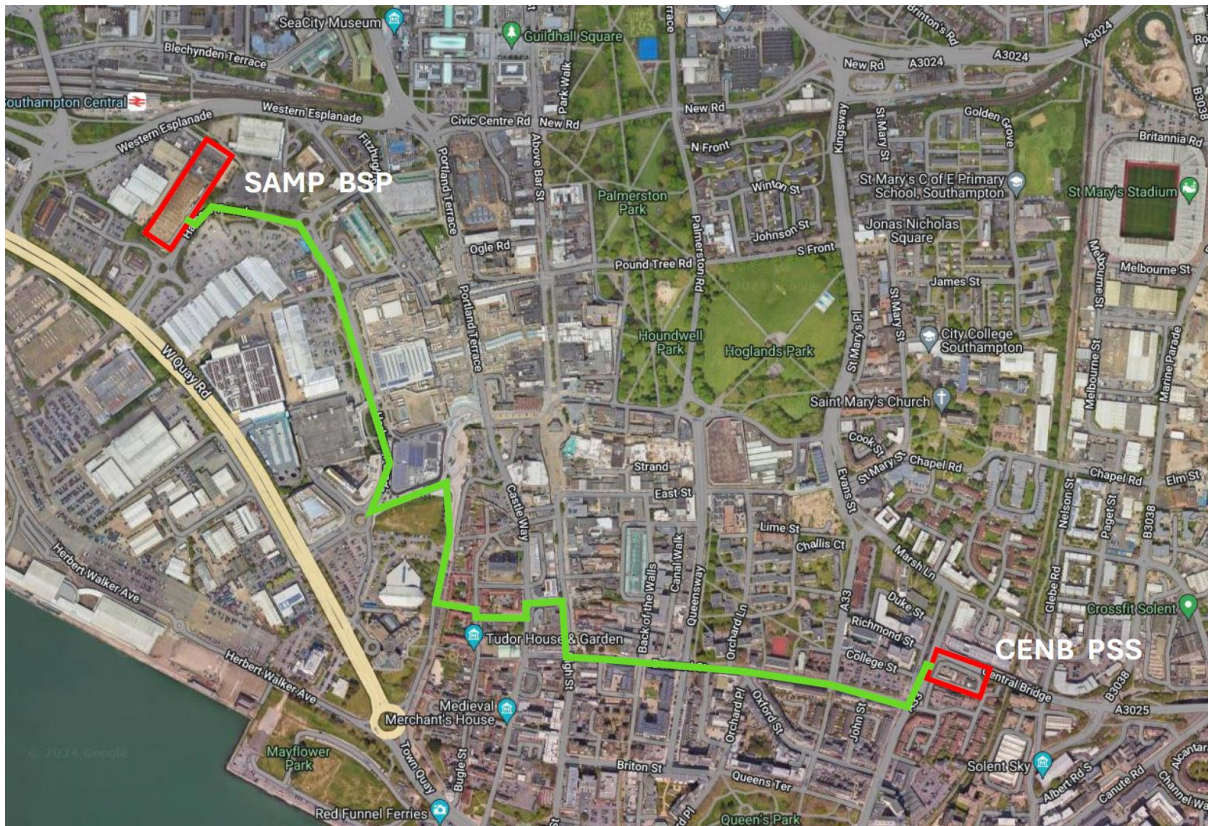
Figure 15: Indicative cable route for the new BSP - Central Bridge underground 33kV circuits
