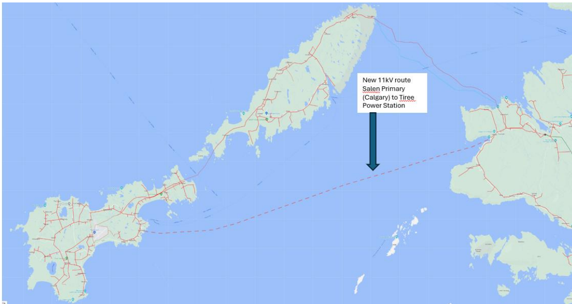
Figure 29 Network schematic with system needs 2041-2050 Option 5 – 11kV subsea from Salen Primary (Calgary).
