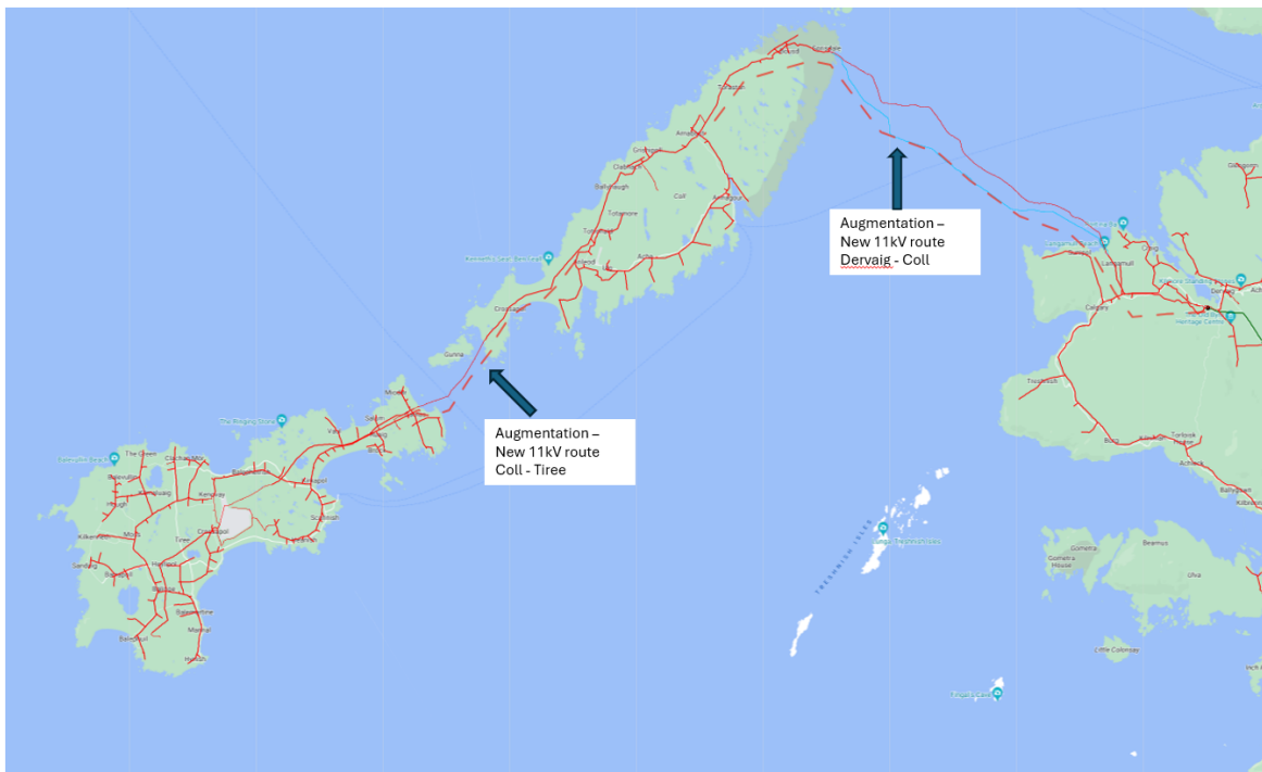
Figure 25 Network schematic with system needs 2041-2050 Option 1 – Augmentation of 11kV subsea.
