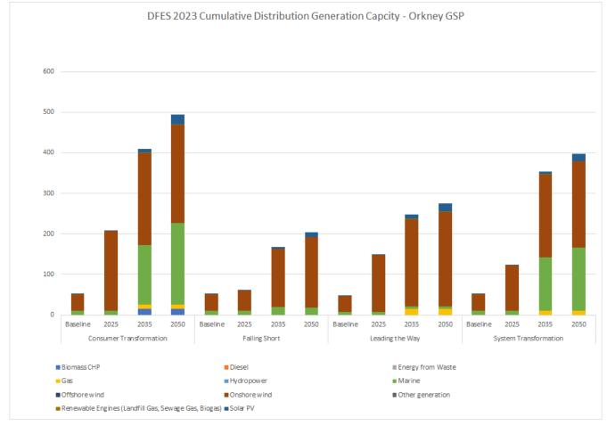
Figure 11 Projected Cumulative Distributed Generation Capacity Orkney (MW). Source: SSEN DFES 2023
