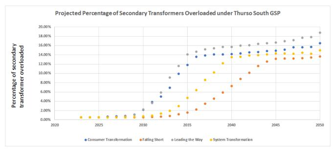
Figure 39 Thurso South Projected Secondary Transformer Loading. Source: SSEN Load Model
