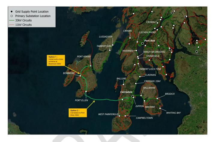
Figure 31 GIS view of network with works in progress and additional reinforcement options by 2028(Options 1 & 2)
