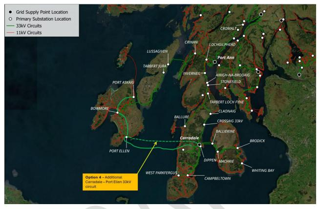
Figure 33 GIS view of network with works in progress and additional reinforcement options by 2040 (Option 4)
