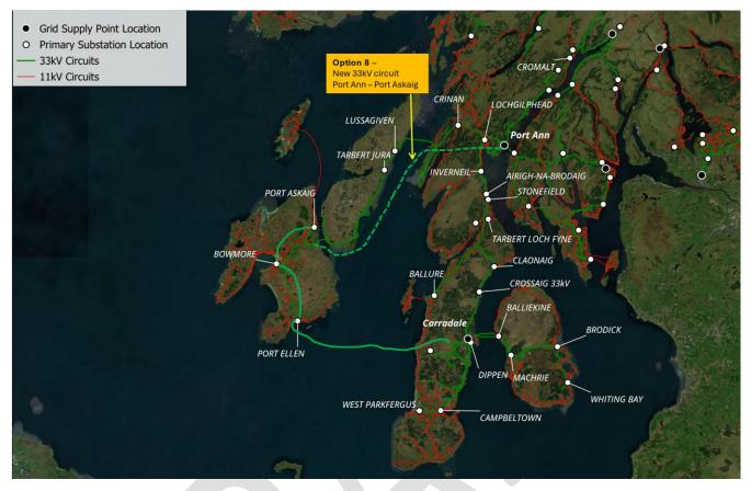
Figure 37 GIS view of network with works in progress and additional reinforcement options by 2040 (Option 8)
